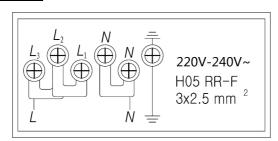
The "Green / yellow" earth wire must be connected to the Earth marked. It must be about 10 mm longer than the live and neutral wires.
