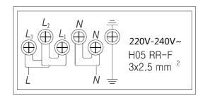
The cable connections must be in accordance with the diagram located on the bottom of the hob.
