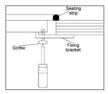
On the underneath of the hob, locate the fixing brackets (B) and turn them so that they locate on the underneath of the worktop and the hob.
